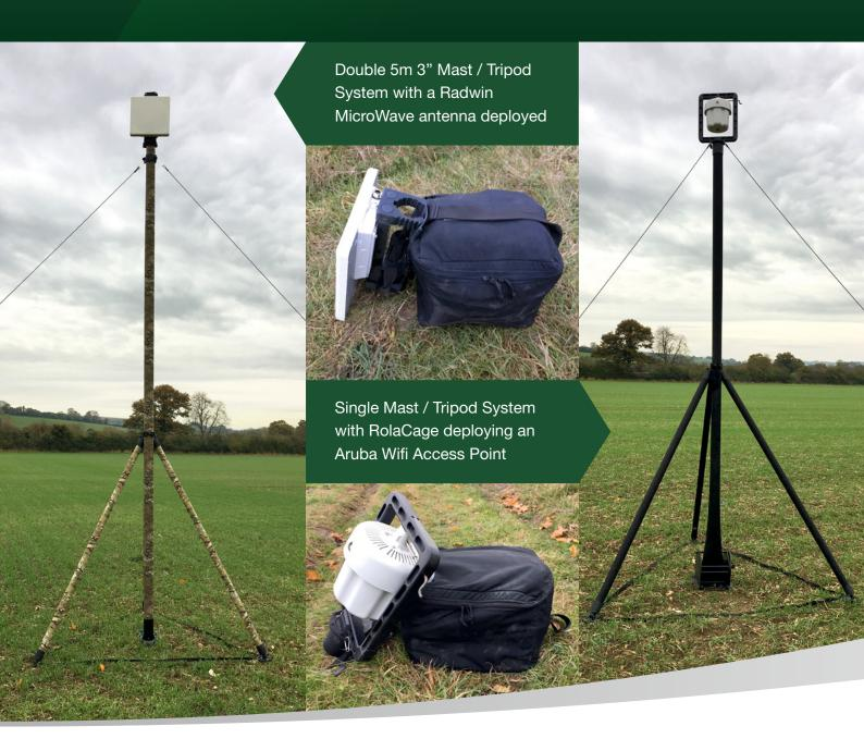
For applications where the tripod system alone does not achieve the desired height for sensor or aerial mounting, REX offers a range of Mast/Tripod combinations that link the benefits of both systems into a single package. Single skin versions can take loads of up to 5kg (11lb), double skin versions can take loads of up to 18kg (38lb).
