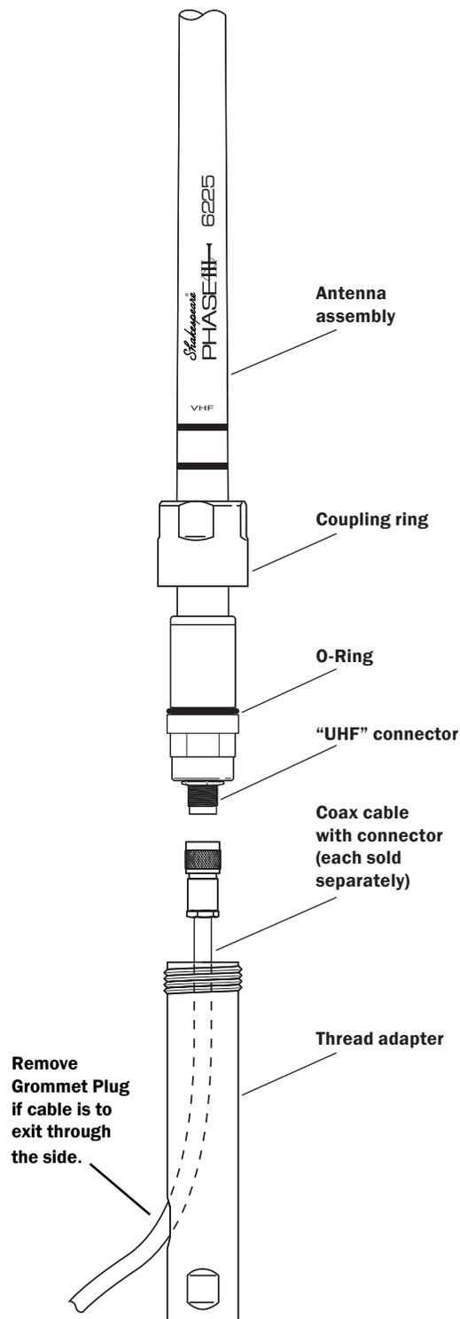
4. Strap the thread adapter to the mast using stainless steel U-bolts, a mast mounting device, or strapping and appropriate hardware (not supplied).
