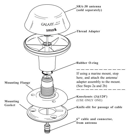
**Step 2:** Route the antenna's cable through the Thread Adapter as shown. Screw the antenna into the Thread Adapter and hand tighten. This assembly, without the
