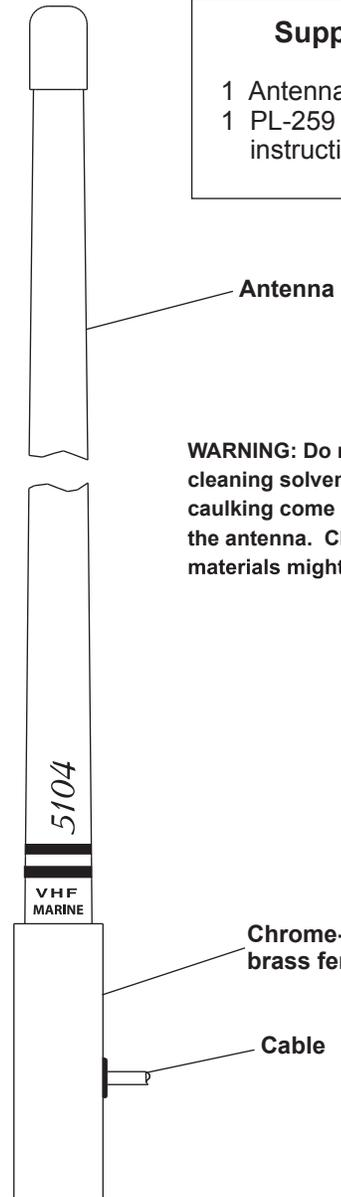
**WARNING: Do not let paint solvents, cleaning solvents, or adhesive caulking come in contact with the antenna. Chemicals in these materials might destroy the finish.**
