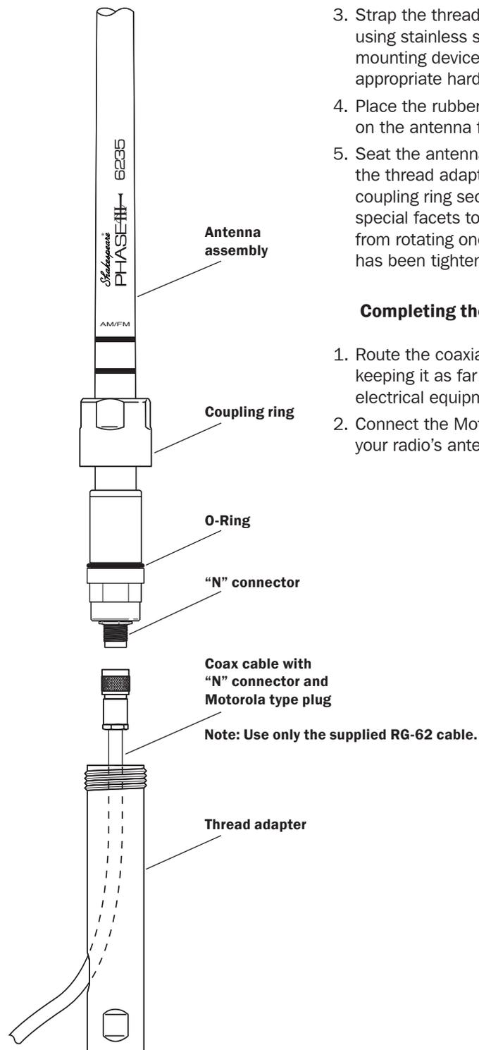
3. Strap the thread adapter to the mast using stainless steel U-bolts, a mast mounting device, or strapping and appropriate hardware (not supplied).
