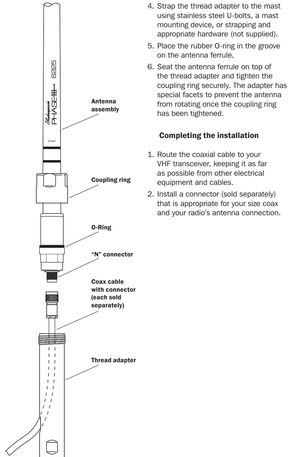
4. Strap the thread adapter to the mast using stainless steel U-bolts, a mast mounting device, or strapping and appropriate hardware (not supplied).
